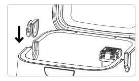
2. Install the removable hose slot plug into one open slot.
